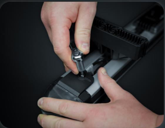
**8.** Secure the endcaps so they are tight against the frame. Leaving a gap between the frame and the light may cause extra wind noise while driving.
