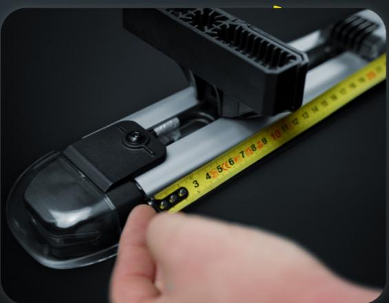
**9.** Measure and ensure the mounting feet are in the correct location. This will vary by vehicle, so we recommend a dry fit on the roof using the rubber feet supplied in the kit. If this step is not performed perfectly, it will leave gaps in the rubber strips.
