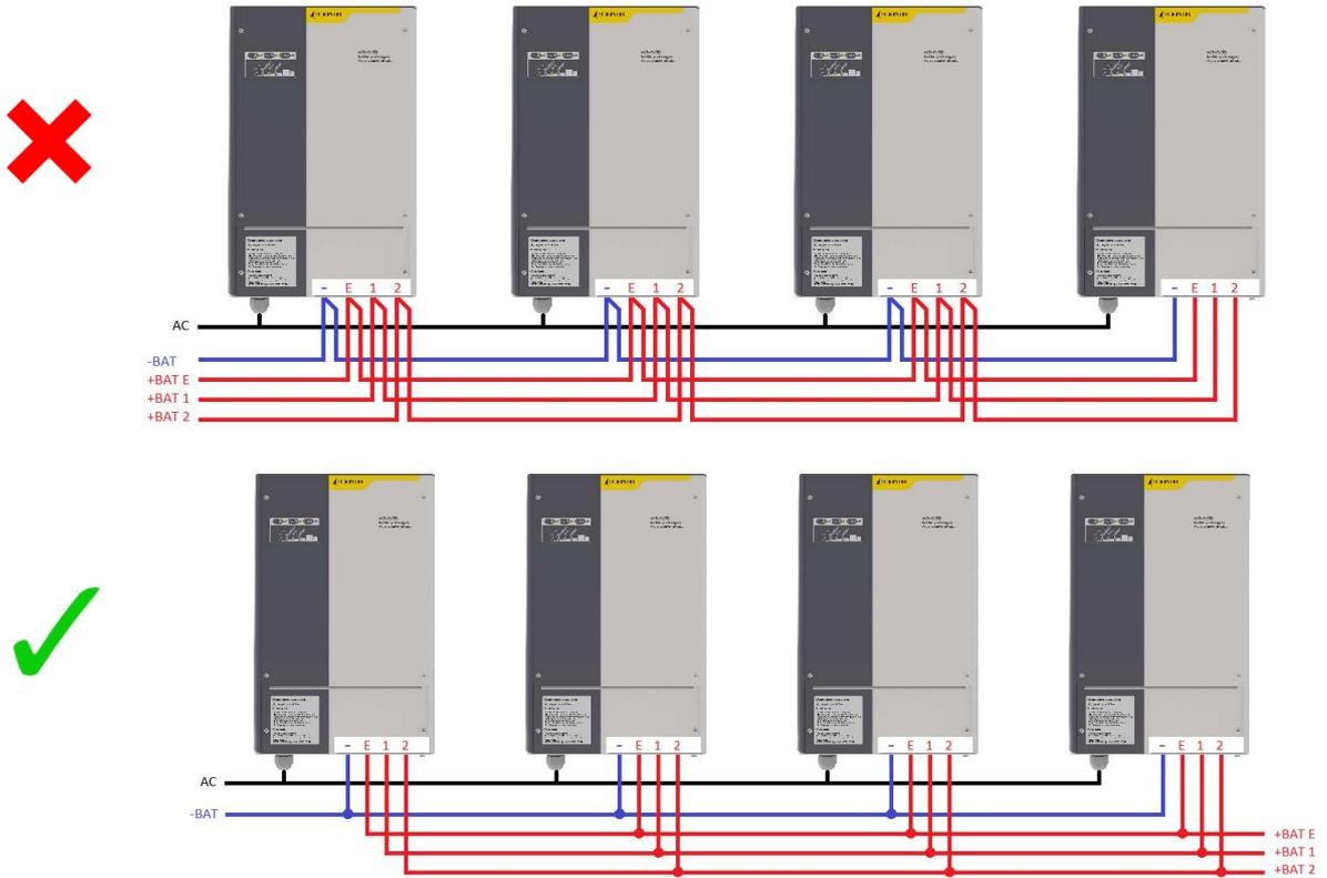
**Step 2 :** Control wiring : the battery charger offers a receptacle matching with connector Phoenix Contact MCV 1.5/4-ST-3.5, 4 circuits (reference 1840382). The cable employed must be insulated. It must be a multi-conductor cable, section 1,5mm<sup>2</sup>. Its length between two battery chargers must not exceed 1 meter. The parallelisation cable and accessories are available as an option.
