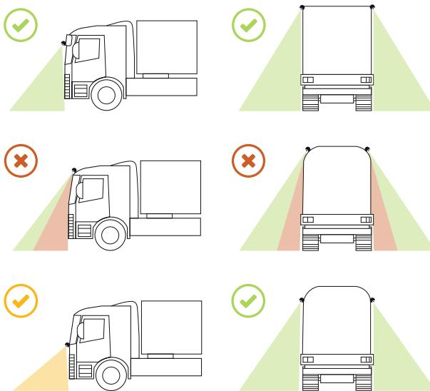
The system limits listed below apply to the mounting positions of the cameras for each side of the vehicle. For calibration, four mats with a geometric pattern are laid out on the floor near the corners of the vehicle. Depending on the camera's mounting height, there is a maximum distance to the outer edge of the calibration mats. Maintaining the maximum lateral distances between the camera and the calibration mats is a prerequisite for successful calibration.
