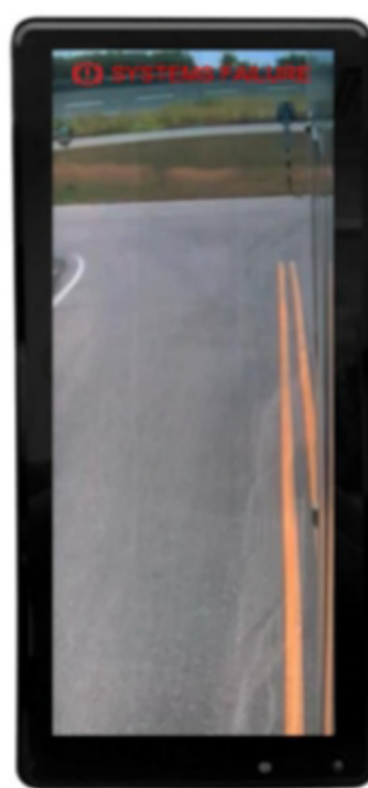
Single camera failed
