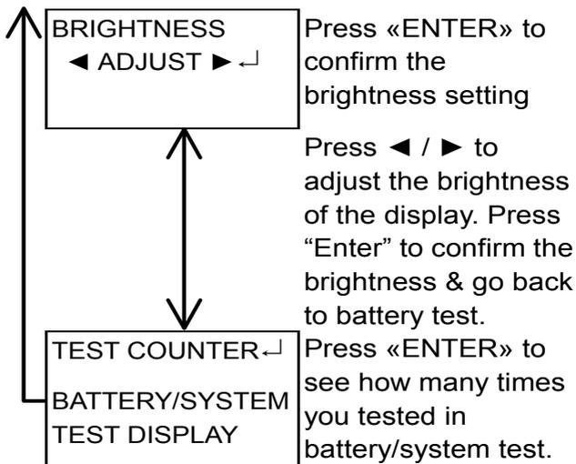
6. Press the ◀ ▶ key to select battery test. Press «ENTER» button.
