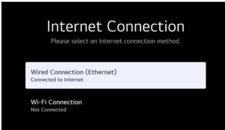
Press ▼ / ▲ button to select Wired Connection (Ethernet). Press **OK** button to enter sub-menu and setup.
