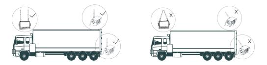
2) Magnet based extension antenna should be attached on the top of the vehicle. Make sure there is no obstacle around or between 2 antennas.
