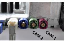
On the back the CA-SCA 3 adapter on the purple connection for camera 1 (rear view camera) or the green one for camera 2
