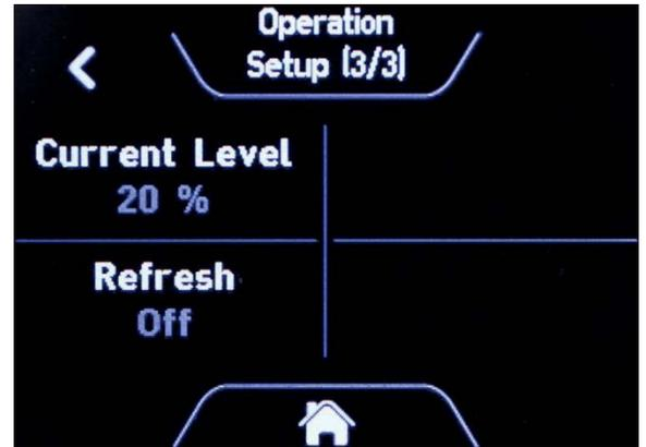
When the HPOWER charger DIP switches are set to A=1, B=1, C=1 and D=1, setting can be selected by the remote display itself.
