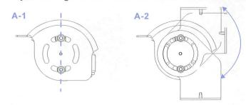
A-1. Recommended guide line for assembling sunvisor. A-2. User can adjust the installation angle.
