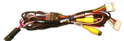
**IN CERTAIN CASES IF THE INTERFACE WILL NOT TRIGGER ON CAN, YOU WILL HAVE TO TRIGGER REVERSE WITH THE GREEN WIRE AND CONNECT TO THE REAR LAMP (12v+)
