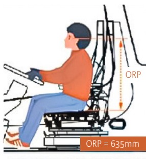
DBC-SV88 Installation reference point
