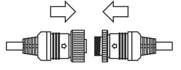
2. Screw the camera connector up clockwise.
