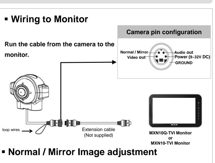
The Normal / Mirror image can be changed via the GREEN loop wire:
