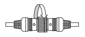
3. Tighten cable connection firmly in order to prevent water ingress.
