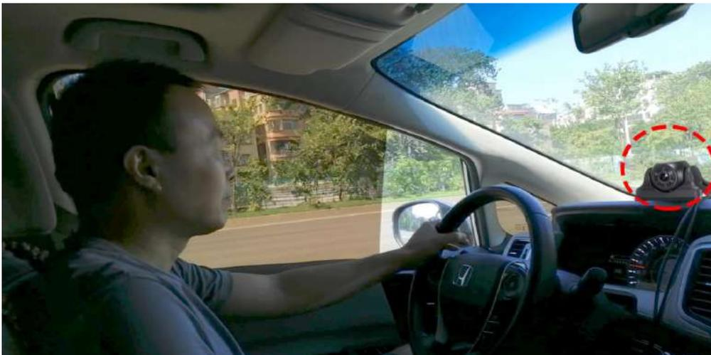
**Calibration:** parameter calibration. Align the face with the calibration frame to conduct calibration. The detection frame is square and blue by default. After the face is aligned with the calibration frame, a green frame will appear on the face. Click the Start button, and pop out a message after 2-3s indicating successful calibration and accompanied by a voice message, click ok to exit the calibration interface.
