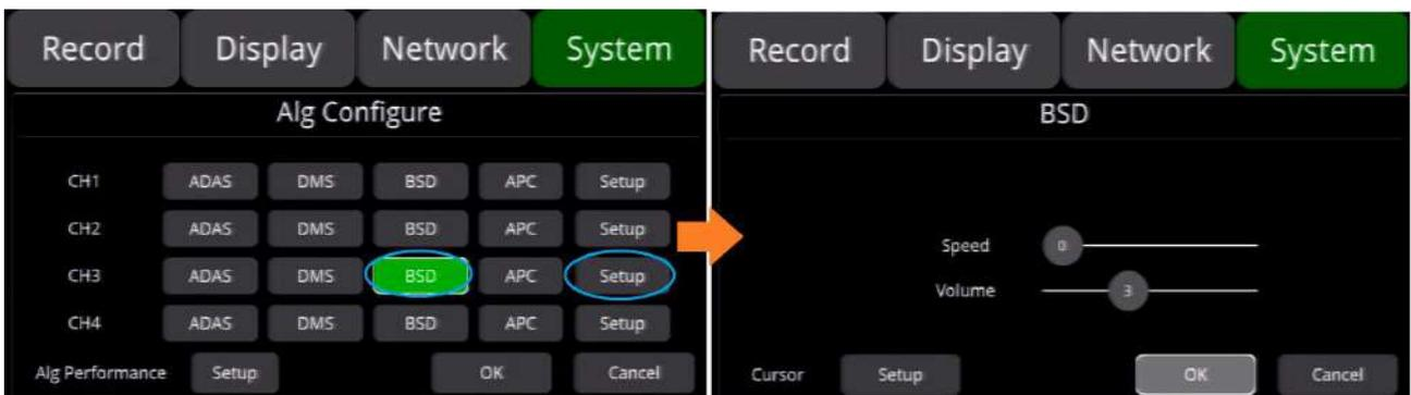
**Speed:** Set the speed threshold for BSD function. When set to 5, the BSD algorithm can be enabled only when pedestrians are walking at 5km/h or above. The default value is 0.
