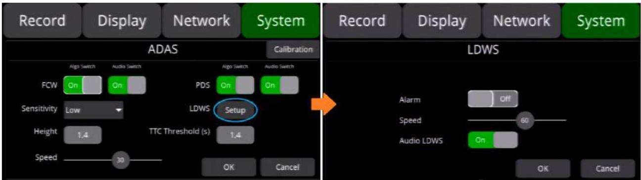
**Alarm:** If it is On, LANE warning will be triggered when vehicle speed is over the setting value and there is lane departure. If it is Off, LANE warning will not be triggered even when vehicle speed is over the setting value and there is lane departure.
