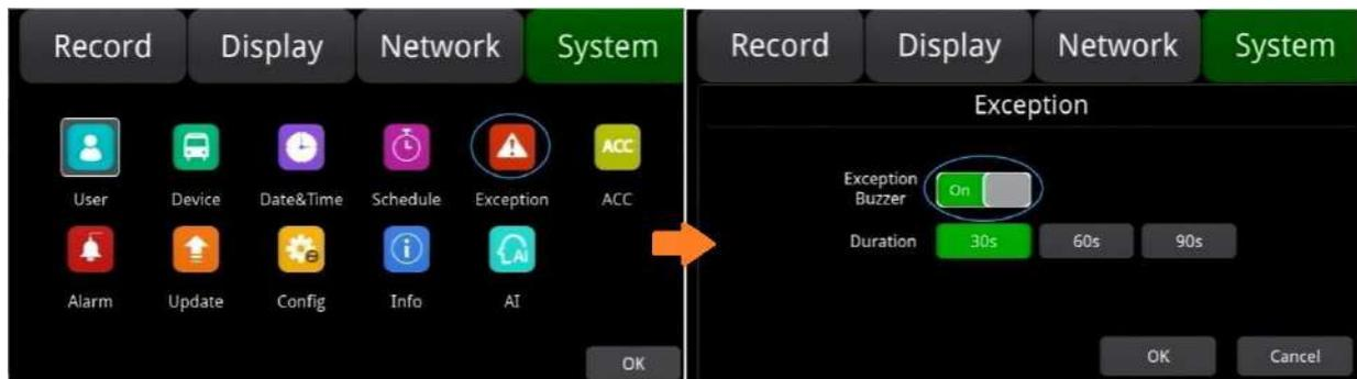
If the buzzer beeps intermittently, it means that the device is unable to record.
