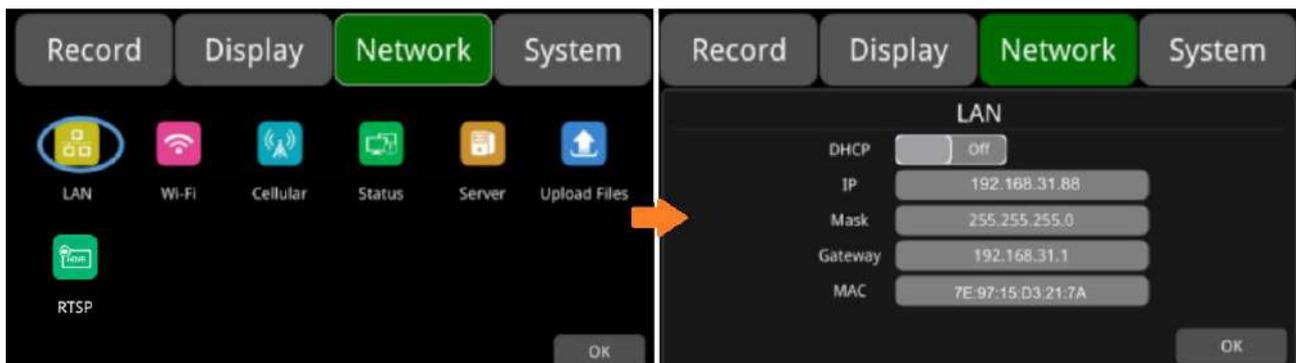
Step 3: If DHCP is set to ON, a dynamic IP will be automatically matched. If DHCP is set to Off, input the IP, mask, gateway and MAC manually.
