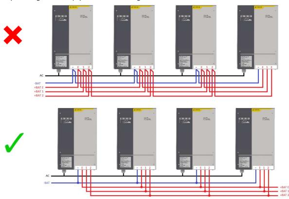
Step 2: Control wiring: the battery charger offers a receptable matching with connector Phoenix Contact MCV 1.5/4-ST-3.5, 4 circuits (reference 1840382). The cable employed must be insulated. It must be a multi-conductor cable, section 1,5mm². Its length between two battery chargers must not exceed 1 meter. The parallelisation cable and accessories are available as an option.
