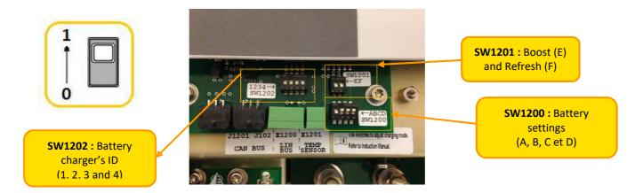
The HPOWER chargers are equipped with switches to configure the charger according the battery type and the application (see section 3.3.2).
