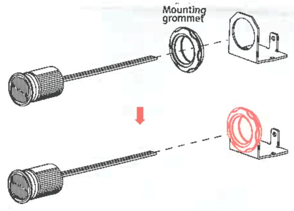
Secure the LIGHTHEAD onto the BRACKET WITH A screw
