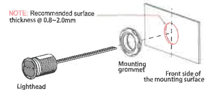
Ensure that the optical stripes are aligned vertically.
