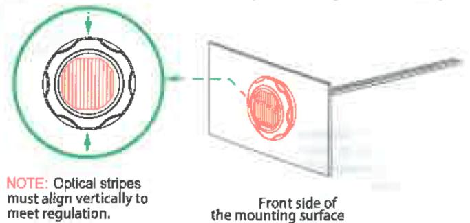
From the front, install the MOUNTING GROMMET onto the cut-out, and insert the LIGHTHEAD.
