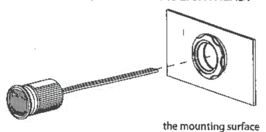
Where necessary, apply silicone around the reverse side to prevent from rotating.
